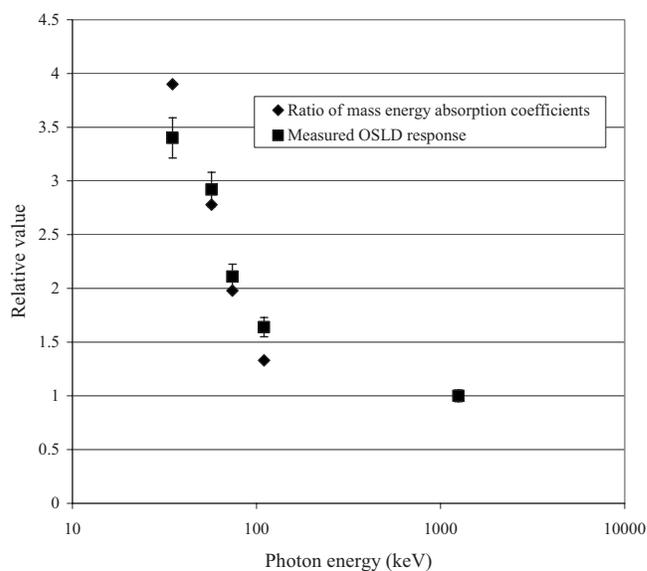
FIG. 7. A plot of the ratio of mass energy absorption coefficients of  $\text{Al}_2\text{O}_3$  to water normalized to their values at  $^{60}\text{Co}$  from Ref. 19 along with the measured OSLD response data from Table I normalized to their response at  $^{60}\text{Co}$  for the kilovoltage energies used in this study. This figure shows that the ratio of mass energy absorption coefficients suggested by Attix (Ref. 18) provide a good approximation of the OSLD response at kilovoltage energies.
